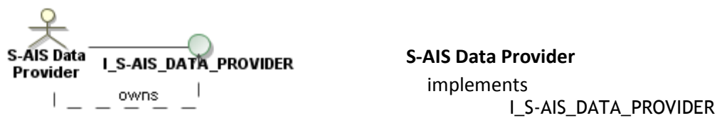
Figure 10 - Interfaces for the S-AIS Data Provider actor
