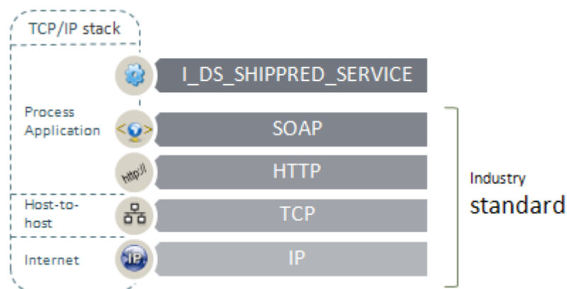
Figure 47 - Protocol stack of the I_DS_SHIPPRED_SERVICE interface
