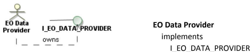
Figure 9 - Interfaces for the EO Data Provider actor
